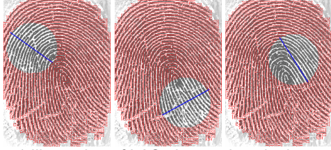
Fig. 1 Illustration of LAS: the sections in the round regions represent their optimized symmetry axes.
