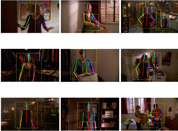
Figure 3. Illustrative results by our model-free discriminative methods with single detection for single person (Left), multiple detection for single person (Middle) and multiple detection for multiple person (Right). The top image of the right column shows that our method can estimate multiple poses for one image at the same time, while the middle and bottom images of the right column illustrate that multiple wrongly-estimated poses caused by over-enlarging bounding boxes for human upper body and localization.
