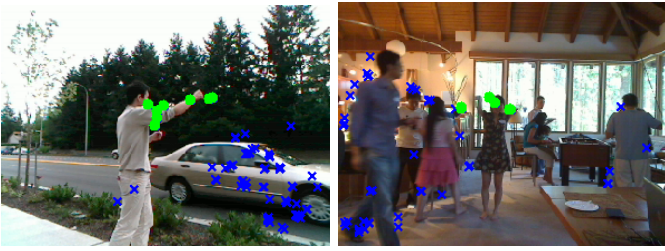
Figure 1. Example video frames in which actions of interest are visually weak compared to ongoing background activity. Dots denote detected interest points which may be relevant (dots) or irrelevant (crosses) to the punching or waving actions.
