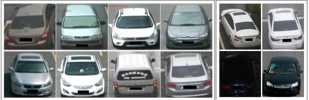
Figure 5: Qualitative evaluations of vehicle model classification. (Left) : Correctly classified vehicle images with large visual appearance similarity between different model classes. (Right) : Misclassified vehicle images due to extreme illumination conditions.
