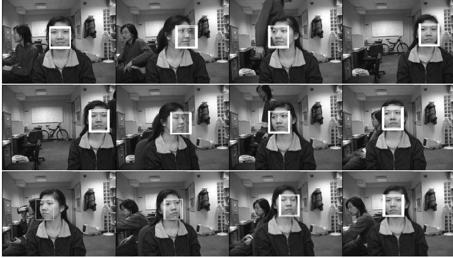
Fig. 1. Experiment 1 - Tracking a non-frontal female face in real-time. The figure shows example images from an indoor sequence (Video Sequence 1).
