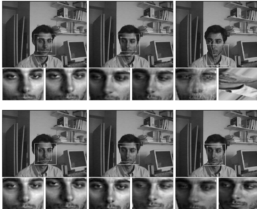
Fig. 6. Top row: EigenTracking without dynamic updating fails due to insufficient training views. Bottom row: The result from using the adaptive scheme.
