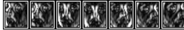
Fig. 12. Templates at 15^\circ intervals used to estimate rotation about the y-axis. The template in the centre is from a frontal view.
