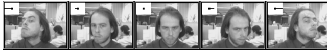
Fig. 13. Tracking and estimating y-axis rotation using the 7 templates of Fig. 12. The needle in the upper-left corner of each image indicates the estimated head rotation.
